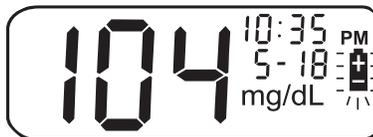
When the battery icon is flashing by itself on the display, **you cannot perform a test**. You must install a new battery before using your meter.
