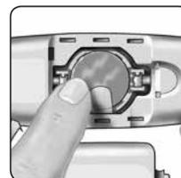
If the meter does not power on after you have replaced the battery, check that the battery is correctly installed with the "+" side up. If the meter still does not power on, call LifeScan Customer Service at 1 800 227-8862 (available 7 days a week, 8 a.m. – 8 p.m. Eastern Time).
