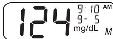
Press ▼ to move to the previous result stored in the meter. Then, press ▲ or ▼ to move forward or backward through all of your results. When you're finished reviewing past results, press and hold ▼ for two seconds until the meter turns off.
