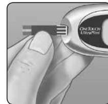
Hold the meter as shown and insert the test strip into the test port. Make sure the three contact bars are facing you. Push the test strip in as far as it will go. **Do Not** bend the test strip.
